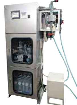
ヨウ素製造工程 かん水中のヨウ素濃度測定 Iodine concentration measurement for iodine production process
